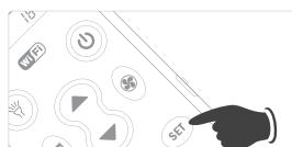
3. Release the SET button **immediately** when the conditioner turns on and check the button functions. If the buttons work correctly, the code setting is effective. If not, please repeat steps 2 and 3.
