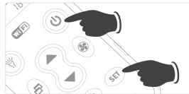
3. Press the SET button to exit, check the button functions. If the device responds correctly the setting is finished, if not, please repeat steps 2 and 3 with next set of codes.
